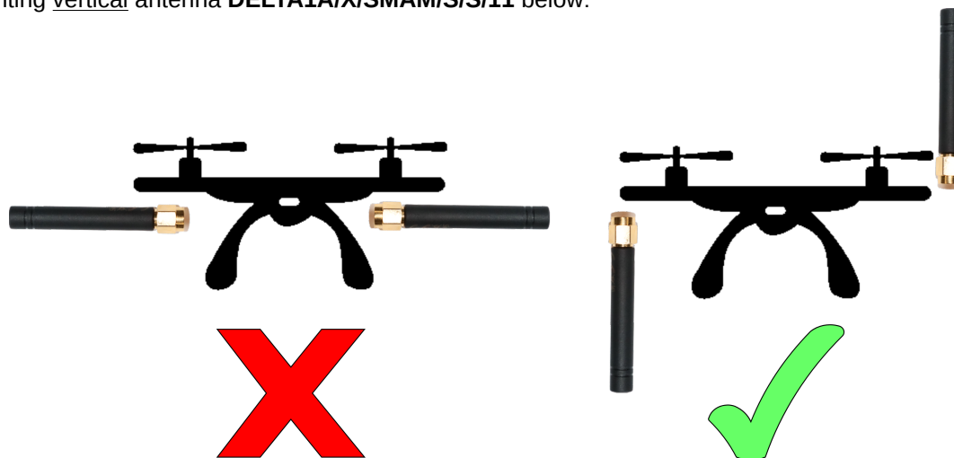
Figure 5: Proper antennas mount
