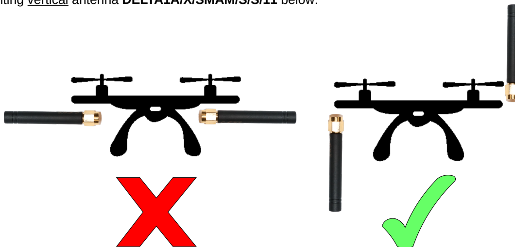
Figure 5: Proper antennas mount
