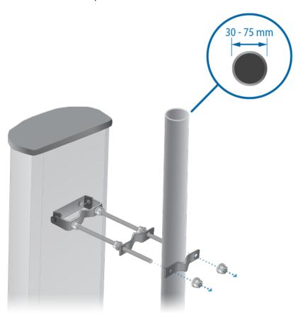
Figure 8: Pole mounting. Source: AM-9M13 Quick Start Guide (www.ui.com/airmax/airmax-sector-antenna/)
