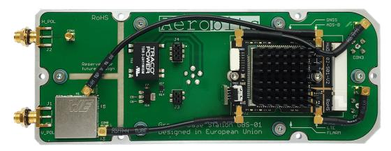
Figure 3: Receiving module without cover
