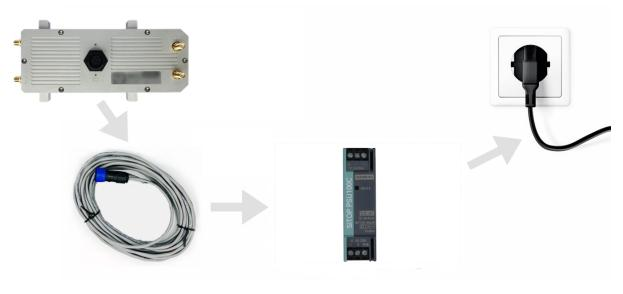
Figure 7: Power supply connection
