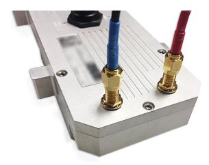
Figure 5: GPS and LTE Antenna cable plug
