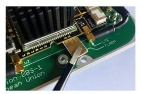
Insert SIM card into slot visible on the picture above. A simple way to do it is to grab SIM with tweezers and push it carefully directly into slot. Then attach the device back (if unmounted) and mount the cover.
